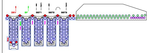
All transport modules (racks) and tanks are designed to reduce chemical oxidation to an absolute minimum. This together with our accurate replenishment, temperature control and constant circulation ensures all processing parameters are maintained within pre-set programmable limits.
