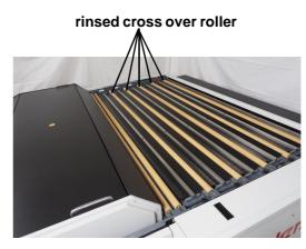
Water rinsed cross over rollers are in place in order to minimize the chemical carry over from one tank to the next as well to keep the cross over section clean and free from any chemical deposits.
