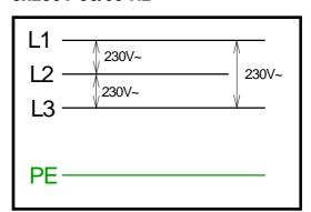
Single phase connection (230VAC - 50/60Hz) is not available for this model!
